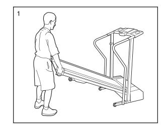
Move your right hand to the position shown and hold the treadmill firmly. Raise the treadmill until the storage latch closes over the catch. Make sure that the storage latch is fully engaged over the catch.
